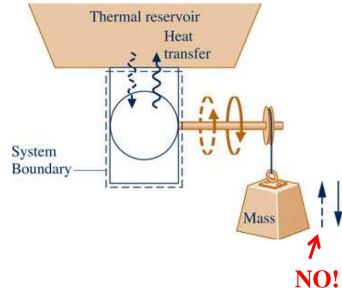
$$W_{\text{cycle}} \leq 0 \quad \left\{ \begin{array}{l} < 0: \text{ Internal irreversibilities present} \\ = 0: \text{ No internal irreversibilities} \end{array} \right. \quad \left( \begin{array}{l} \text{single} \\ \text{reservoir} \end{array} \right)$$
