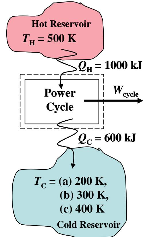
**Solution:** To determine the nature of the cycle, **compare** actual cycle performance ( $\eta$ ) to maximum theoretical cycle performance ( $\eta_{\text{max}}$ ) calculated from Eq. 5.9
