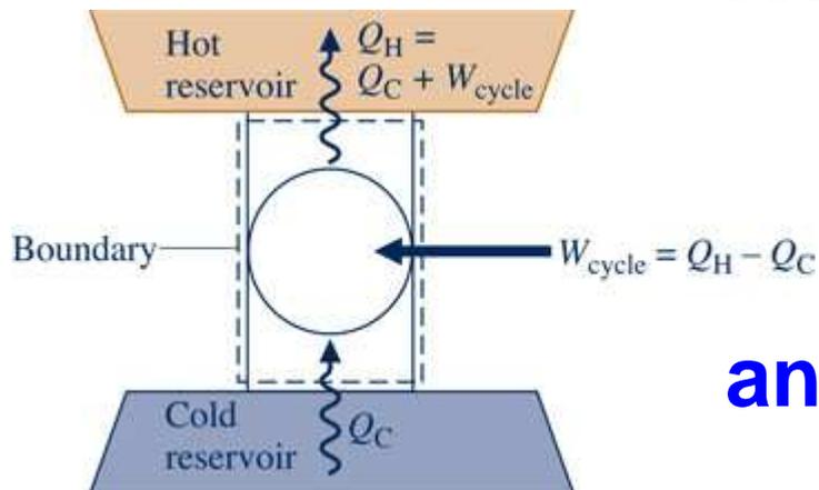
$$\beta = \frac{Q_C}{W_{\text{cycle}}} = \frac{Q_C}{Q_H - Q_C} \quad (\text{Eq. 5.5})$$
